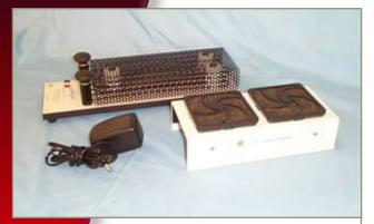
uildline 9230A series of precision DC current shunts are true 4-terminal devices intended for the precise measurement of DC current. They are constructed from specially selected elements supported on an insulating base for mechanical stability and covered with a perforated metal cover to allow proper cooling while providing physical protection for the elements.
